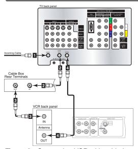
Figure 2. Connecting VCR with cable box.
